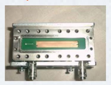
In order to facilitate the repair of the anodewire, the wire is mounted on a stable FR4-carrier, which can be easily exchanged.
