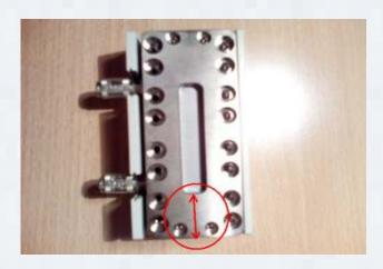
Distance from detector outline to active detection region has been reduced down to 20 mm. This is especially important in the case of cascading detectors, e.g. for SWAX measurements. The 'blind gap' between detectors is reduced to a minimum.
